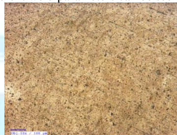
(b) AA 2014, Speed-1100rpm, Feed-30mm/min
