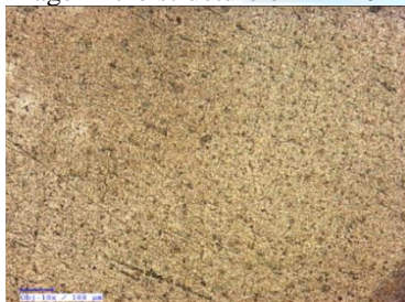
(a) AA2014, Speed-900rpm, Feed-20mm/min,
