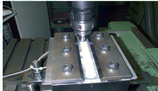
Fig: 2 Friction stir welding process
